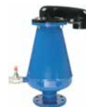
Series 701/78 Combination air valve Orifice sizes: Automatic: 16 mm 2 Kinetic: 5024 mm 2 Steel Inlet flange PN 16 DN80-200
