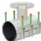
Series 729/32 Repair clamp Double band with flanged branching and fingers Stainless steel AISI 304 or AISI 316 NBR or EPDM rubber
