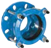
Series 603 Supa® flange adaptor Universal for cast iron, ductile iron, steel, uPVC and asbestos cement pipes Ductile iron DN40-400
